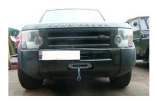
Prior to removing parts from your vehicle fit the winch into the mount.
