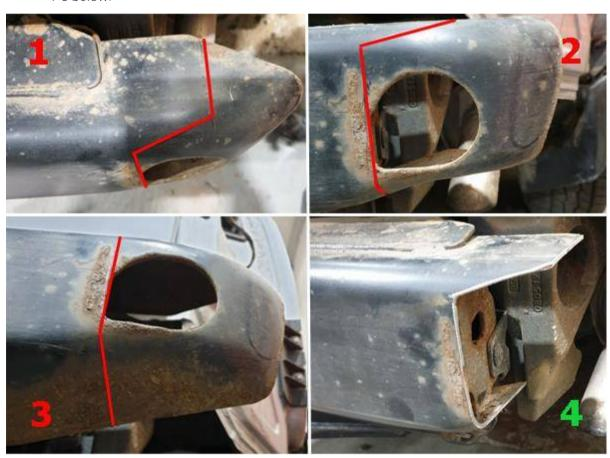
Cut carefully with an angle grinder ensuring you protect glass and body work against sparks. Once cut dress the cut edges (image 4) and protect with an anti-corrosion paint/spray.
