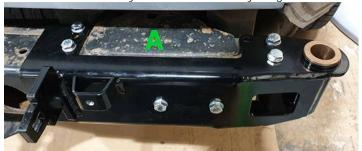
Drill and bolt holes 1 using captive nut plates as supplied. Once holes A are fully tightened then drill and bolt the rest starting at the top. Holes under neath also have a captive plate.
