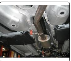
Remove (8) nuts and (10) bolts using a 10mm socket to remove the plastic underbody panel and lower bumper cover fascia.
