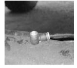
Fit the new 90° fitting into position on the axle ensuring that it is fully tightened down. Push the 6mm pipe into this, once secure it should not be easily removed unless the blue ring is depressed at the same time.
