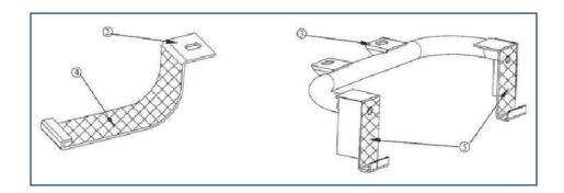
2. Prior of installation, protect the areas which the brackets mount to so you will not scratch the paintwork.
