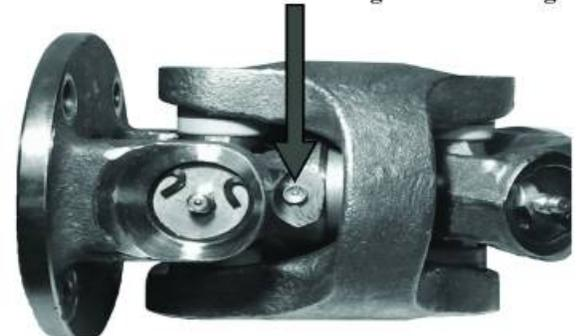
If you have a grease fitting in your CV, it will be a small flush type fitting which is concaved and has the check ball in the center. Greasing this type of fitting will require a special adapter on your grease gun such as the Plews-Lubrimatic # 05-019. The end of this adapter will have a conical point, when pressed against the check ball on the grease fitting, which will allow grease to enter the CV.
