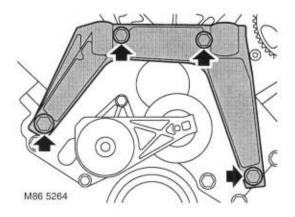
Remove 4 bolts securing engine mounting bracket to engine front plate and remove bracket.
