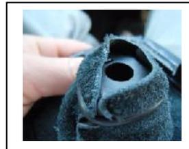
2. Remove parking brake boot by pushing down near the top to release flexible frame- you will have to bend the frame slightly but it is meant to do that so that it "snaps" in place. Once the frame is released, you will turn the boot inside out so that you can get to the grommet. Once you take the grommet off, it should just slide right off.
