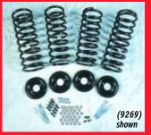
valve blocks, and no more stiff ride! You get the replacement springs and all the required hardware and step-by-step instructions at a fraction of the cost of a new air system. (You'll like the ride better, too!)
