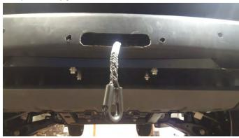
LR4 Winch controller adapter, for Warn winches (LR3 is flat and is installed on driver-side of engine bay)
