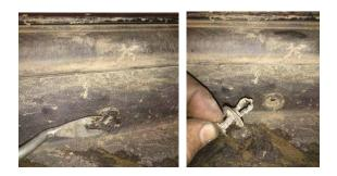
3. Remove the 10mm nut from the centre of the lower section at the rear of the front wing; the plastic trim should now be free to be removed. Trim off the excess thread from front wing mounting bolt.
