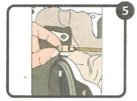
After you have recorded these parameters. You can now remove the 10mm nut at the end of the rod and the two at the actuator bracket.
