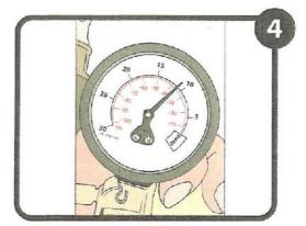
When disc is properly closed you should not be able to turn the disc. With the flapper disc snug against housing, you can now record the in. Hg reading of on your vacuum pump gauge.
