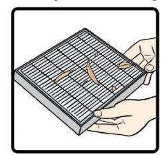
While the air intake is off, it should be properly cleaned or replaced. Ensure no debris enters any of the turbo housings or oil feed/drain to prevent premature turbo failure.
