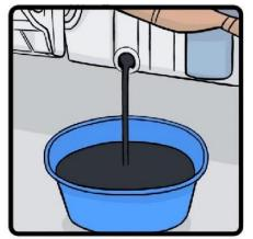
1. Prior to installing new turbocharger, the old motor oil and oil filter must be drained and properly disposed of. A new oil feed line and oil filter must be installed with your new turbocharger to validate warranty.
