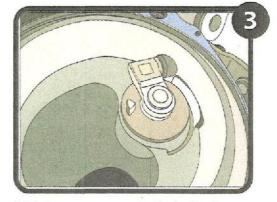
With the vacuum pump attached to the nipple, record how many pumps in takes to close the flapper disc.
