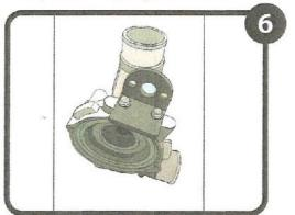
Proceed with the installation of the original actuator/bracket to the new TPC turbocharger by repeating the previous steps. Make sure all nuts and bolts are secured properly after installation of new parts and turbocharger.
