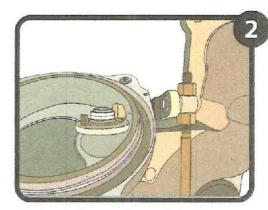
Waste gate flapper disc starts in the open position from factory (2014-2017).
