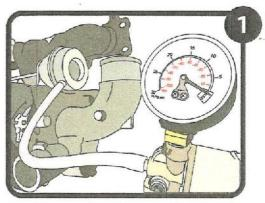
Install vacuum hand pump to the original actuator's nipple like in illustration.
