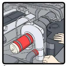
**3**. Once turbo has been installed and all pipping connected, you must now do a "Boost Leak Test". A "Smoke Test" is acceptable with prober smoke machine. Testers must be installed at the turbo inlet when possible. These tests ensure your turbo systems is free of any turbo destroying air leaks.
